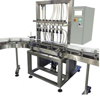
Overflow Filling Machines provide a fill to a level system, or cosmetic fill, which works well with products that vary in viscosity or where container interior volume may vary slightly. The level fill is also ideal for products packaged in clear containers, boosting shelf appeal. Typical products include distilled spirits, water, edible oils, sauces, lubricants personal care products, household chemicals and more!
